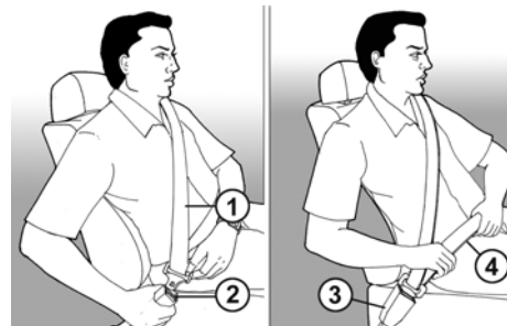
1. Seat Belt 2. Tongue 3. Lock Buckle 4. Lap Belt
