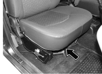
Jack & tools location (Below driver's seat)
