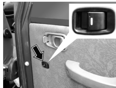
Individual Switches on the rear doors for operating the rear door glasses
