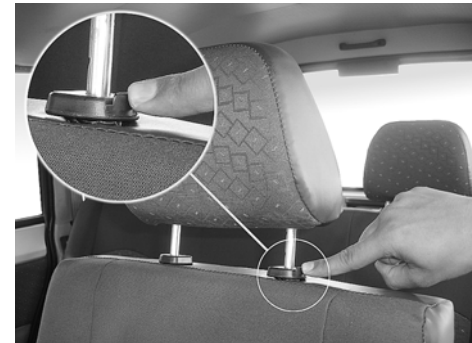
Release Button for Head rest height adjustment
