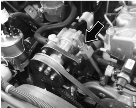
Power Steering Pump Belt Adjustment Nut
