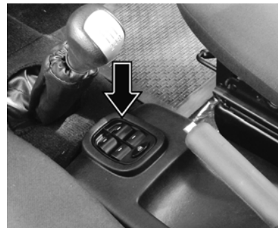
Switches on the central console for operating the door glasses
