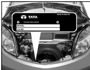
Chassis Number Plate mounted on front cross member, below bonnet
