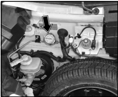
Location of CNG pressure gauge
