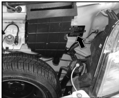
CNG compliance plate location
