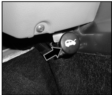
Location of hood release lever
