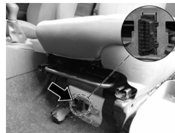
OBD connector below co-driver seat
