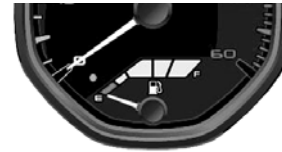
Fuel Gauge (Diesel)
