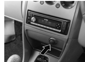
Front Power Socket ( on central console )
