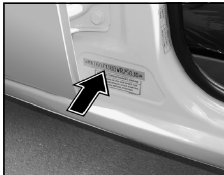
Chassis Number on 'B' pillar
