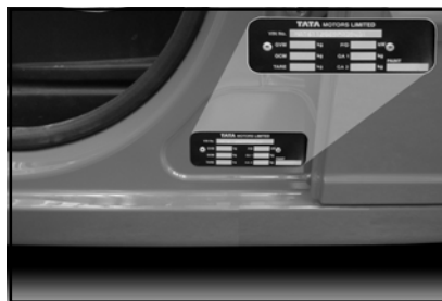
CHASSIS NUMBER ON LH 'B' PILLAR
