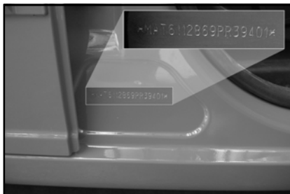
CHASSIS NUMBER ON RH 'B' PILLAR
