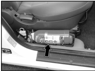
Location of Fire Extinguisher
