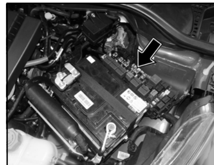
Fuse Box - Engine Compartment
