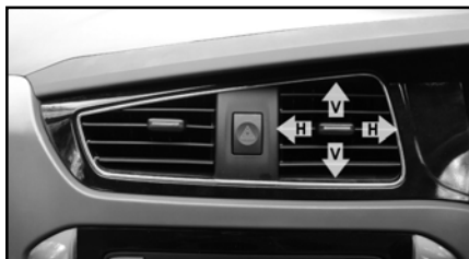
Middle air vent
