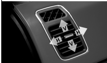
Side air vent
