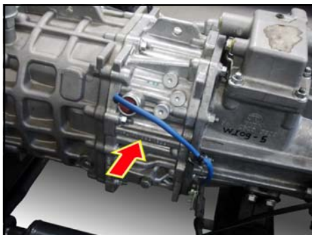
Gear Box Number - Punched
