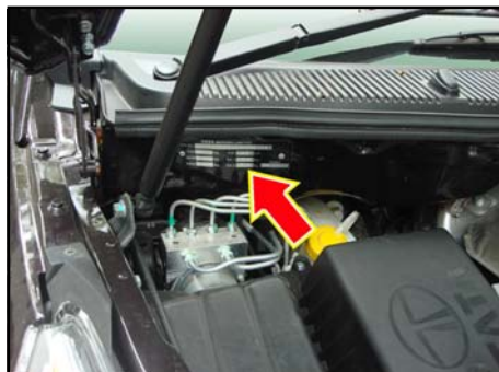
VIN Number Plate (Near ABS Unit)
