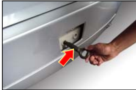
Tow Hook Attachment Location at Rear
