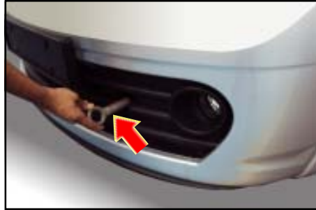
Tow Hook Attachment Location at Front
