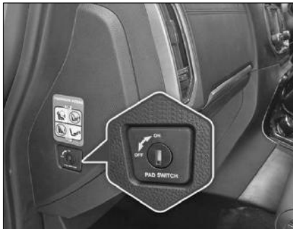
PAB deactivation switch
