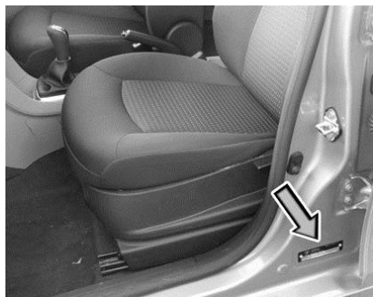
VIN plate near front passenger seat
