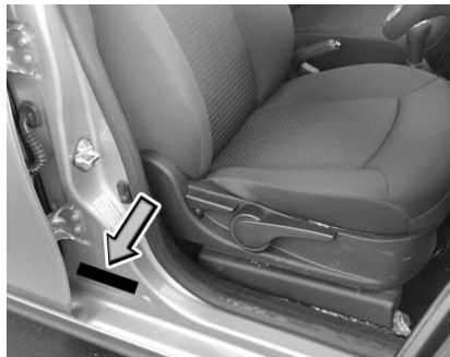
Chassis No. punching near driver seat
