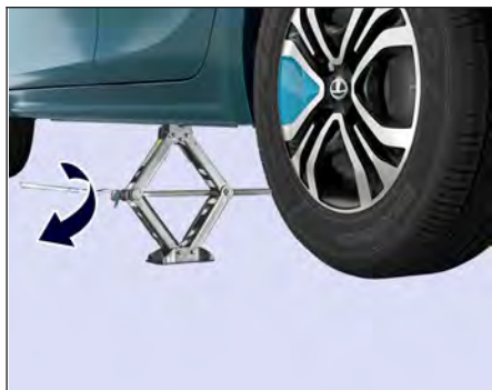
Lifting the front wheel using jack
