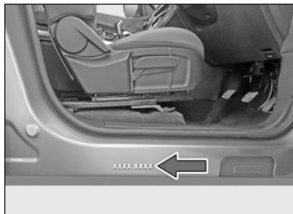
Chassis No. punching near driver seat (RHS outer side)
