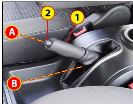
1. Parking brake lever 2. Release button A. Parking Brake Applied Position B. Parking Brake Released Position
