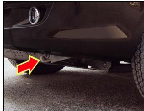
Tow Hook Attachment Location at Front
