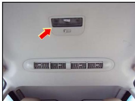
Roof lamp for second row seat passengers (Mounted above 2nd row seat)
