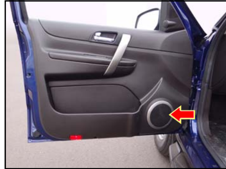
1. Speaker on front door 2. Tweeter in the inner cover of ORVM
