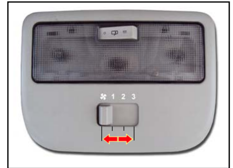
Rear A.C. blower speed control switch
