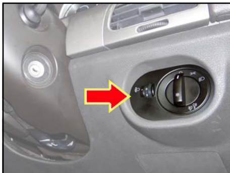
Location of master light switch
