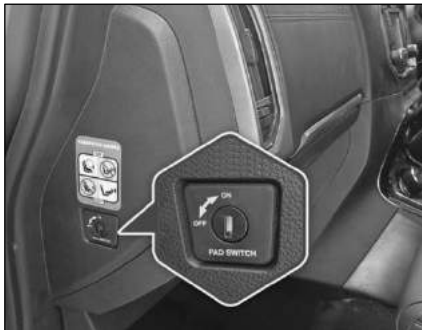
PAB deactivation switch
