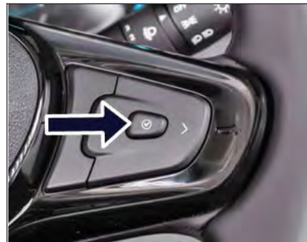
Steering control which needs to be used for Selection of iTPMS Reset
