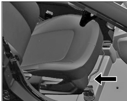
VIN plate below driver seat
