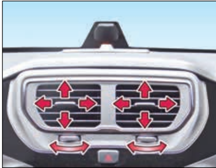
Center air vents
